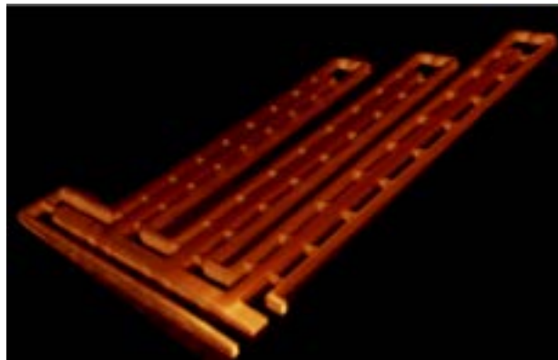
▲ Figure 2: (left) 3D X-ray of the fabricated multiplexer structure; (middle) full-wave simulation of the structure's E-field intensity; (right) measured device response across the 220-330 GHz band.
